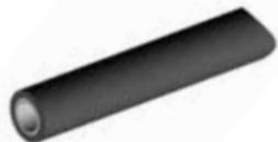
2. Cut and remove the jacket from the tubing to the proper length for insertion into the jacketed tube connector. Refer to the table for jacket cut lengths.
