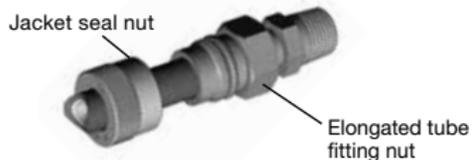
2. Tighten the jacket seal nut hand-tight. The jacket seal nut will cover the vent O-ring when it is sufficiently tightened. If desired, perform a *pressure decay* leak test.
