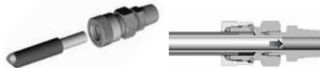
6. Mark the elongated tube fitting nut at the 6 o'clock position.
